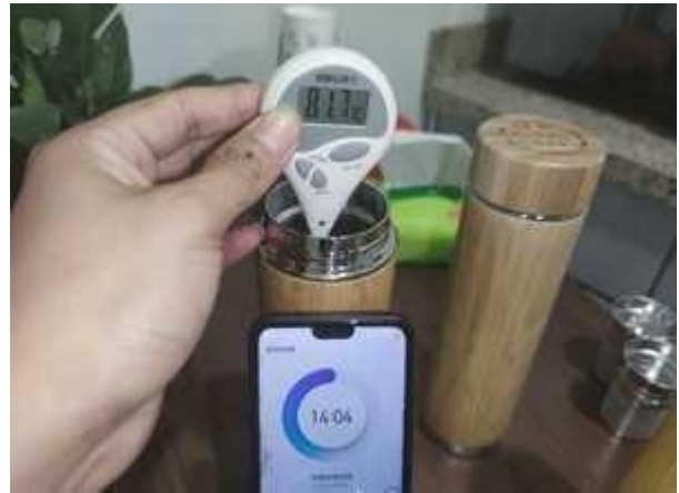
P-086 Thermal-retention check - after 1 hour (2/4) Original source report page 20 of 26
