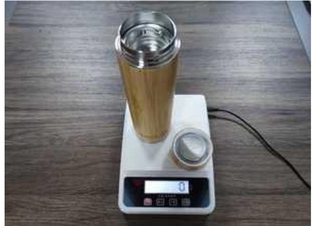
P-074 Usable-capacity check - 1 pc - 480 ml - PASS (1/2)
