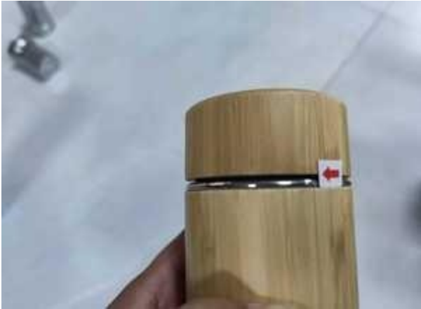
P-047 Oversized visible gap - minor - 3 pcs (3/3) Original source report page 12 of 26
