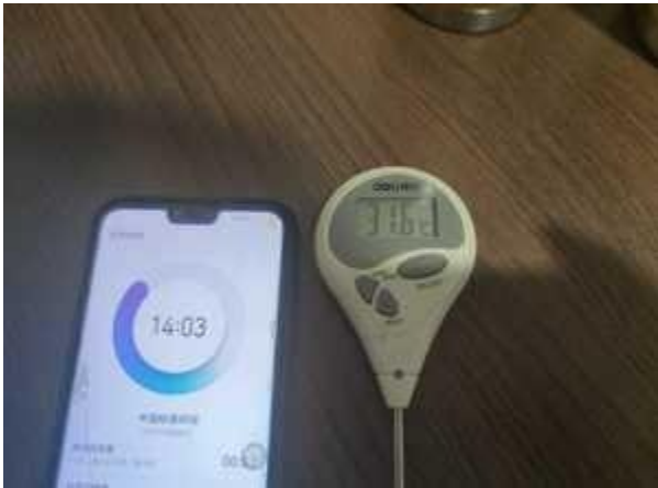
P-085 Thermal-retention check - after 1 hour (1/4) Original source report page 20 of 26
