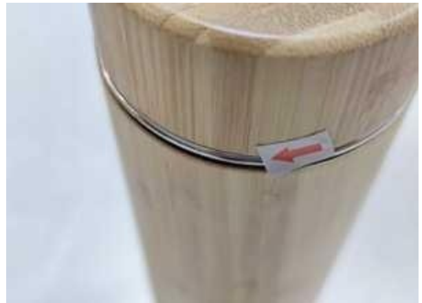
P-052 Localized clearance gap - minor - 2 pcs (2/2)
