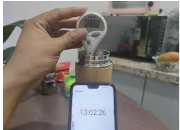
P-082 Thermal-retention check - 3 pcs - start (2/4)
