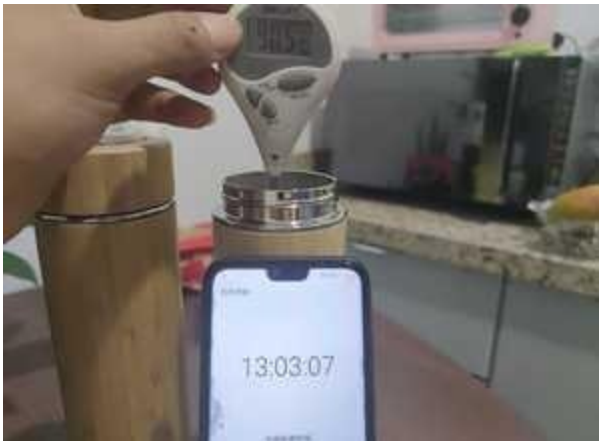
P-083 Thermal-retention check - 3 pcs - start (3/4)
