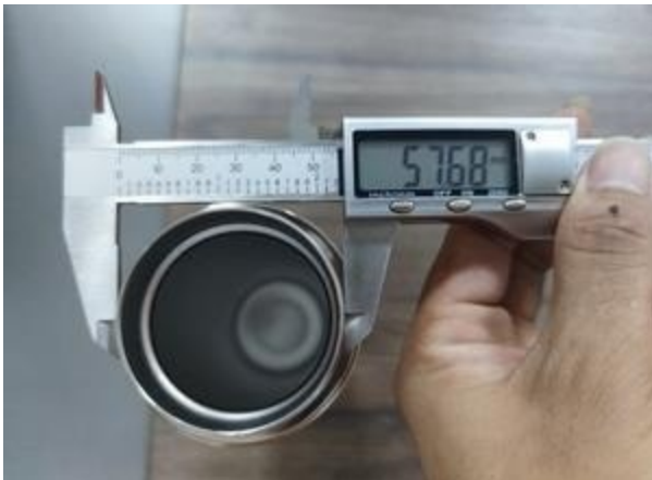
P-067 Outside opening diameter 57.68 mm Original source report page 16 of 26
