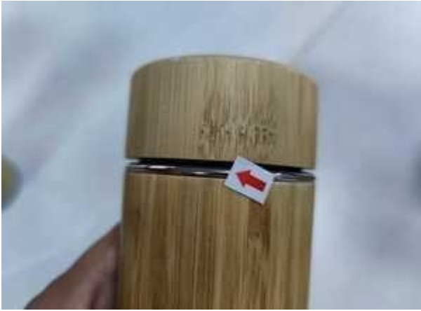
P-045 Oversized visible gap - minor - 3 pcs (1/3) Original source report page 12 of 26
