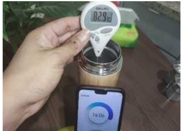
P-088 Thermal-retention check - after 1 hour (4/4) Original source report page 20 of 26
