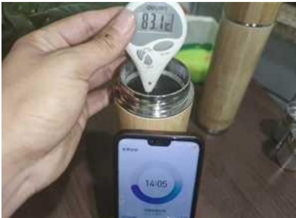
P-087 Thermal-retention check - after 1 hour (3/4) Original source report page 20 of 26
