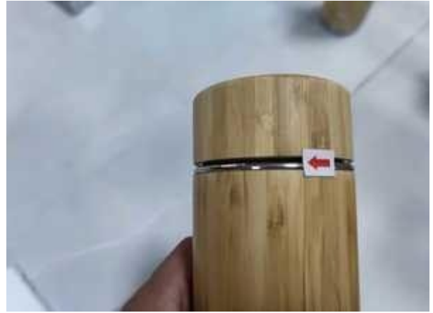
P-046 Oversized visible gap - minor - 3 pcs (2/3) Original source report page 12 of 26
