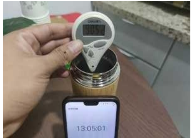
P-084 Thermal-retention check - 3 pcs - start (4/4)
